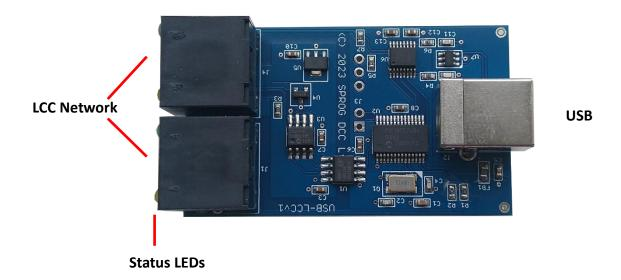
Four status LEDs are built in to the network connectors. One indicate USB activity, one indicates LCC power is present, and two configurable LEDs that default to LCC message send and LCC message receive.
