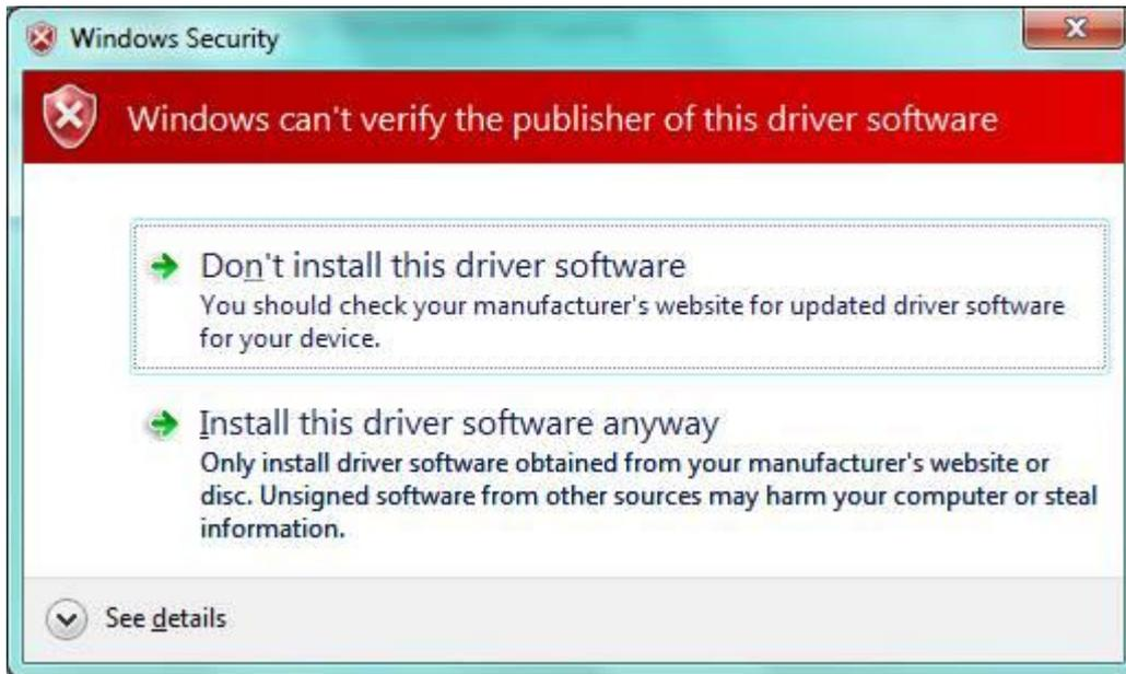
The base drivers are fully compatible with Windows7, and those supplied on the CD are the latest drivers. To make them SPROG II specific, the .inf files are edited which, unfortunately, causes this dialogue to appear.
