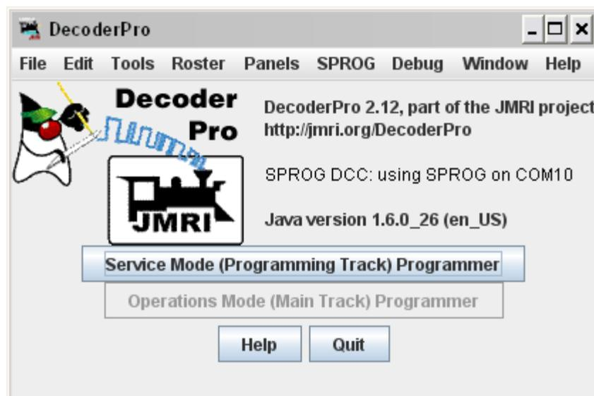
Click “Service Mode (Programming Track) Programmer” to open the Programmer Setup window. A new window will pop up which shows a list of decoder manufacturers.
